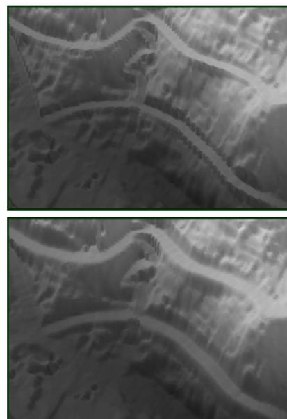
Figure 2: Section from the DTM Stuttgart; resolution 1 m; top: streets broadened around middle axes, bottom: bordering regions adjusted with linear interpolation within a given buffer zone.
