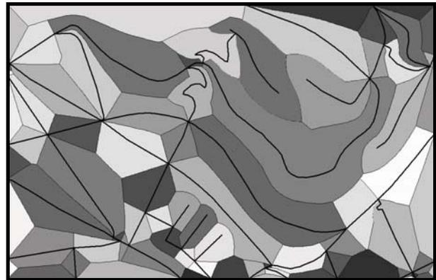
Figure 4: Voronoi cells (in different grey scales) calculated with *VRONI* (Held, 2001), for the street segments (represented by black lines) for a section of the city of Stuttgart.
