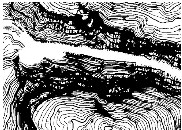
Figure 2. Typical example of problematic area for contour vectorization from contour map layer
