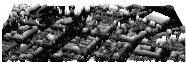
Figure 2 – 3D view of the laser scanner survey
