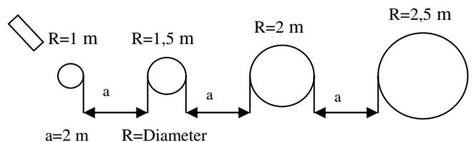
Figure 1, Location and sizes of ground control points
