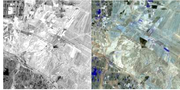
Figure 2. Panchromatic IRS-1C image (left), and ASTER original bands of B_1 , B_2 , B_3 in RGB format
