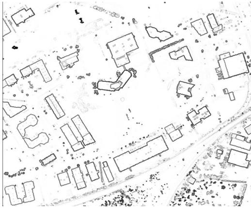
**Figure 3:** Delineation of buildings using shaded relief on the LIDAR elevation data
