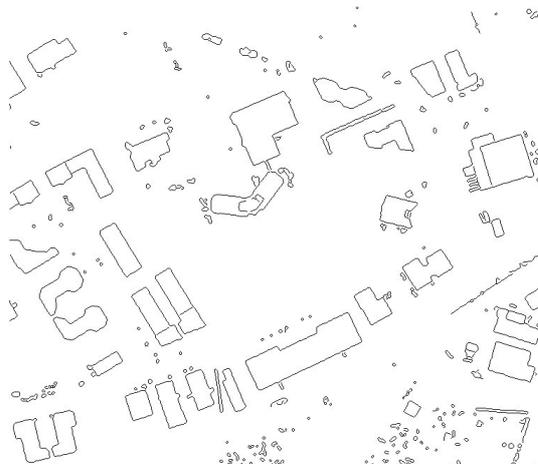
**Figure 4:** Delineation of buildings using Canny edge detector on the LIDAR elevation data
