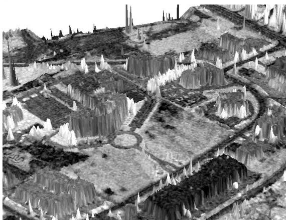
**Figure 5:** Intensity image draped over LIDAR DSM
