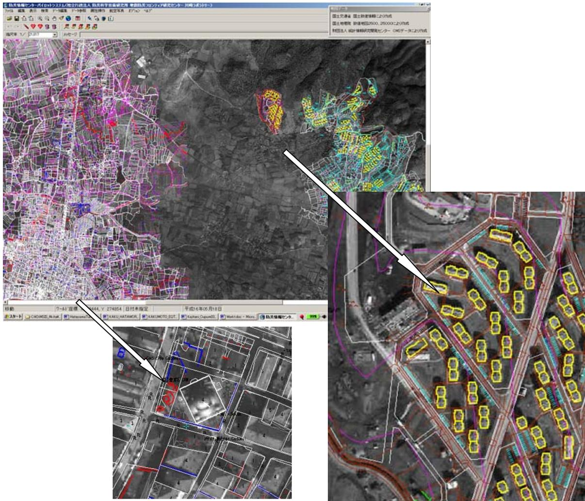
Fig10. Quickbird image data and integrated vector data
