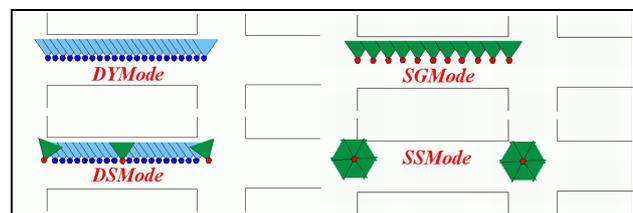
Fig.4: CityGrid Acquisition Modes (Left: Camera/Scanner Modes; Right: Pure Scanner Modes)
