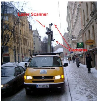
Fig.5: CityGrid Scanner at work
