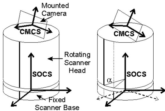
Fig.1: Scanner and Camera Coordinate System
