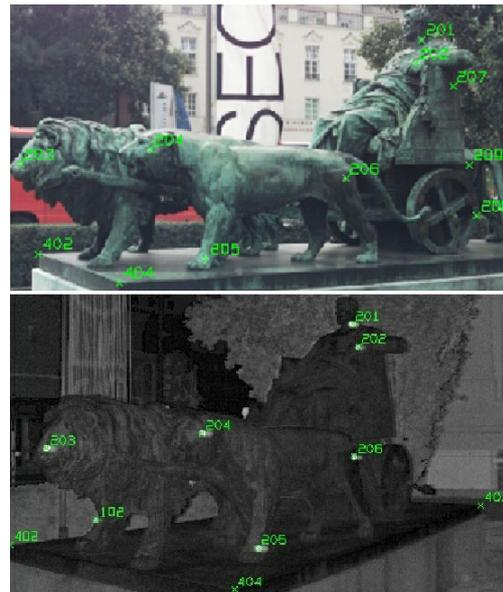
Fig.6: Marc Anton monument (Above: Kodak DCS image. Below: Laser intensity image). Retroreflecting tie point targets are numbered.
