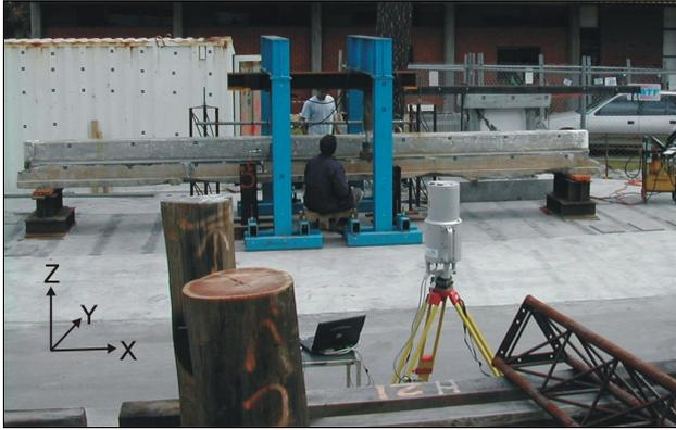
Figure 2. Concrete beam and the Riegl LMS-Z210.
