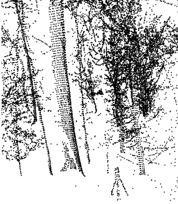
Figure 1: Point cloud of one scan. To improve visual appearance, the point cloud has been thinned out by averaging points in a  $10 \times 10 \times 10 \text{cm}^3$  raster. The scanner was positioned on the right side of the image in the background (not shown), yielding a view on the inner side of the trunks.
