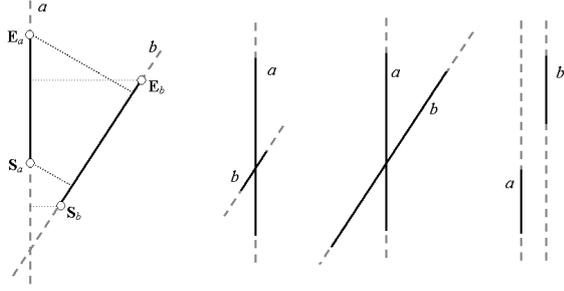
Figure 3: Measure of alignedness: The distance between two segments  $a$  and  $b$  is the mean distance of the distance of the start and end point of either segment to the line carrying the other segment (dotted lines). The three examples on the right side are used to demonstrate properties of this distance measure.
