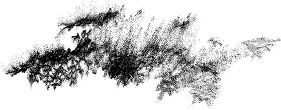
Figure 4: Example of laser scanner point cloud of a branch on a coniferous tree. Scattering of the points in the top-to-bottom direction in the image can partly be caused by the wind, other possible sources are the mixing of ranges to targets within one laser beam.
