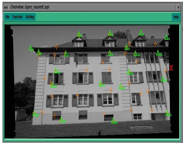
Figure 2. Measured Control Points for exterior orientation
