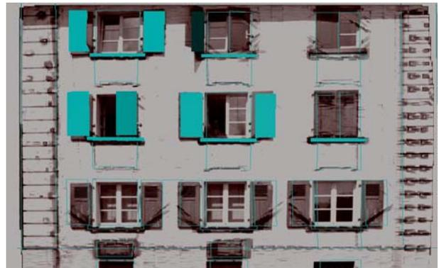
Figure 12. Overlapping orthophoto and 3D photogrammetrical design
