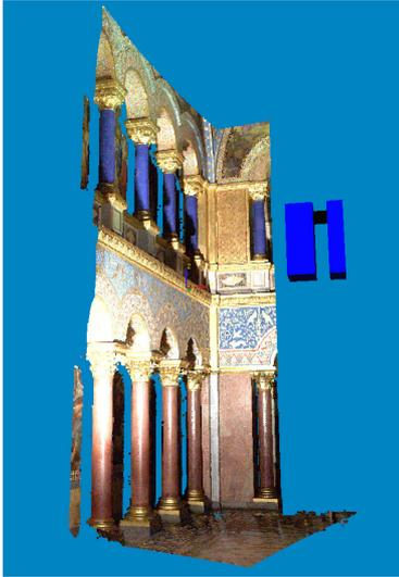
Figure 10: The figure shows a part of the drawhall of castle Neuschwanstein as colored 3D point cloud.
