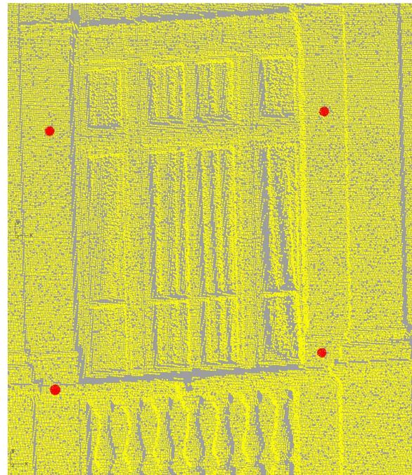
Figure 14. View of the central window (multiresolution scan) with the common targets
