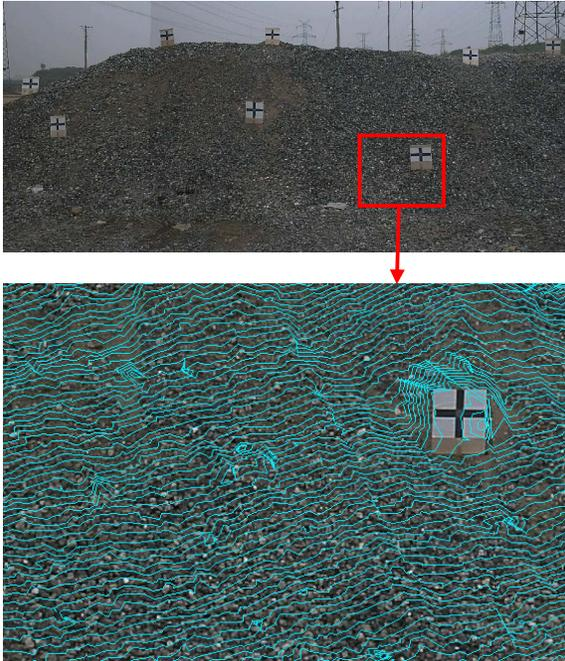
Fig. 5 PTSS has been used to measure stone pile.
