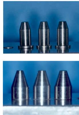
Figure 2. Shoulder and knife-edge abrasion
