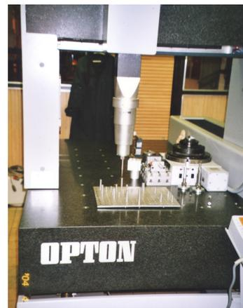
Figure 5. The calibration of the test field with a Zeiss 3D coordinate-measuring instrument
