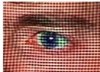
Figure 4: Top: The ShapeCam system consists of a flash projecting a grid and a camera. The camera takes an image from a direction that is slightly different from the direction of projection. Bottom: A regular square pattern is projected on the scene, as seen in this detailed view. 3D co-ordinates are calculated for all the line intersections, resulting in the simultaneous measurement for thousands of points.
