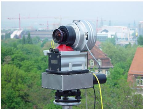
Fig. 3: Digital panoramic camera EYESCAN M3
