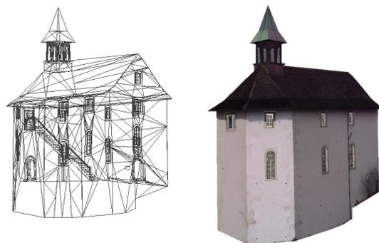
Figure 3: CAD model and fully textured 3D model of the chapel of Zwingen
