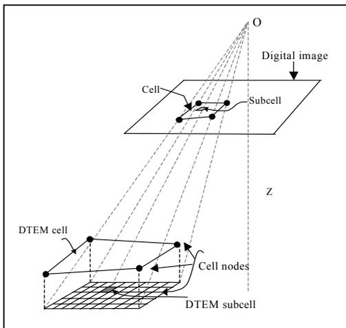
Figure 3. Projection and densification of the DTEM
