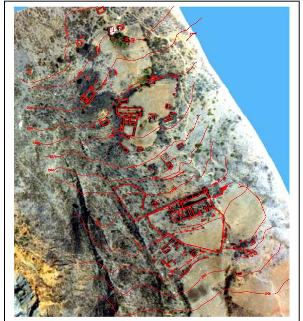
Figure 13. Digital orthophoto with restitution superimposed
