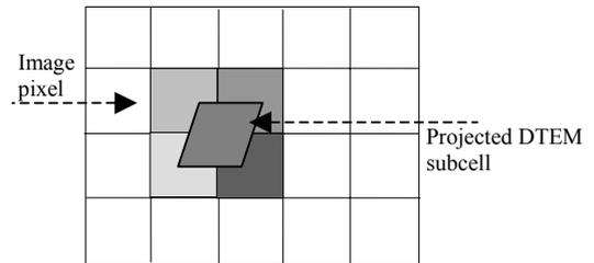
Figure 4. Projection of the DTEM subcell on the digital image
