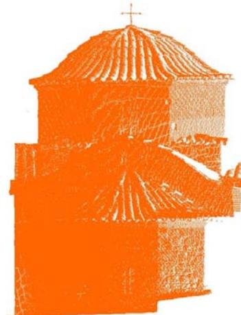
Figure 3b. Snapshot of the merged point cloud from the eastern facade of the church (data set II)
