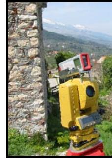
Image 2: First integration-development of GTS 211 D REFLECTORLESS total station with Disto laser in 1996.
