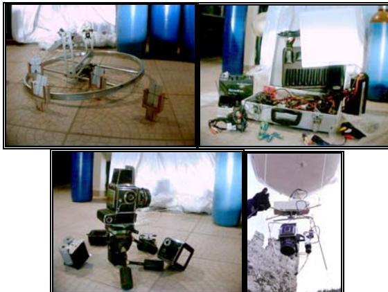
Image 4: The 3-axis radio-controlled base, the gases fuelling cylinders, the video telemetry system, the semi-metric Hasselblad 25-ressau camera and the balloon.
