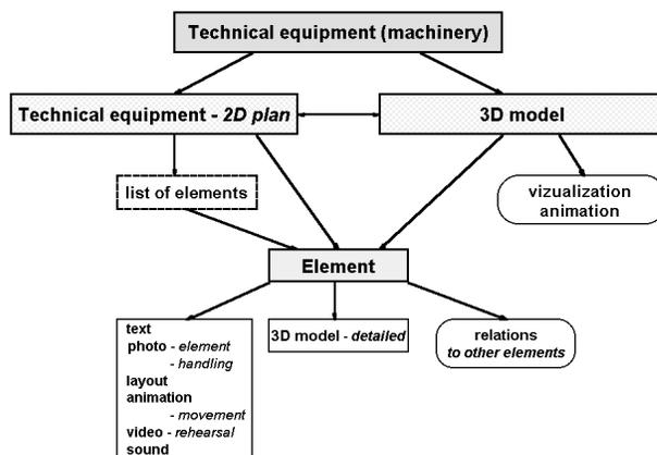
Chart 7. Scheme of data, subsystem – research of site, element of technical equipment
