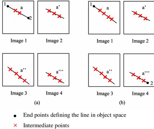
Figure 2. Schematic drawing representing two scenarios for the selection of the end and intermediate points in overlapping images
