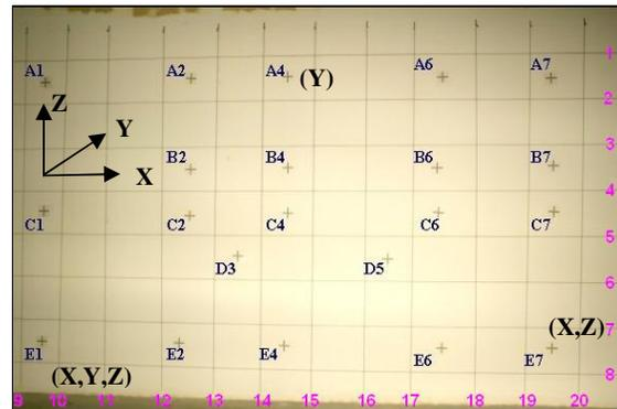
Figure 3. Calibration test field with 20 lines and 21 points
