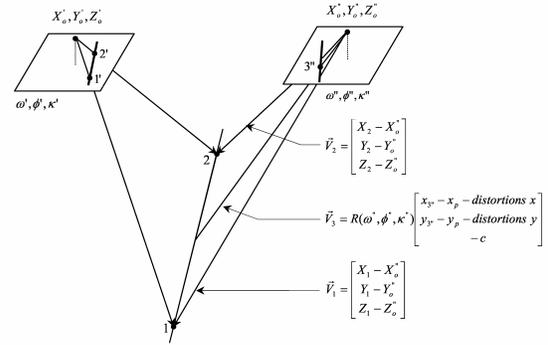
Figure 1. Perspective transformation between image and object space straight lines
