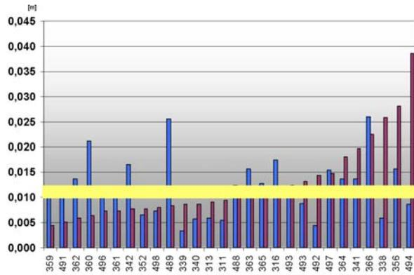
Table 4. Comparison between natural points, topographically measured, and the same ones on the surface model
