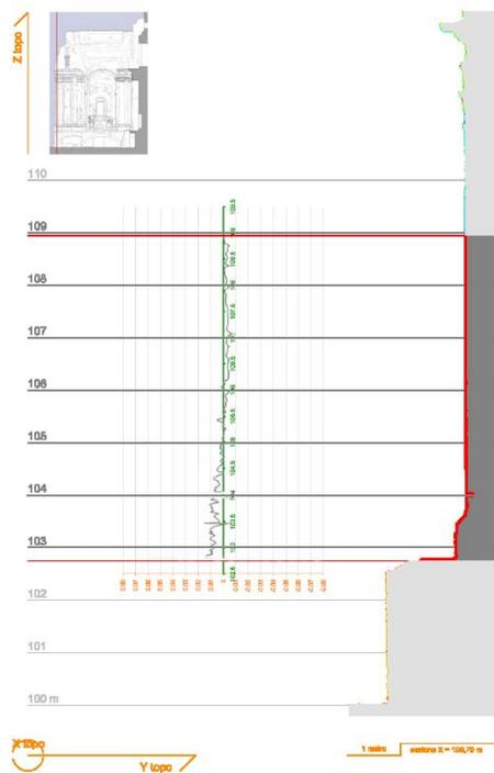
Figure 12. Graphic representation of the comparison, carried out with the above mentioned program, between the photogrammetric sections and the corresponding sections on the registered cloud of points
