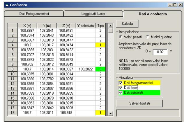
Figure 11. Screenshot of the program for comparison between photogrammetric section and the “strips” of points extracted from the cloud: Residuals  $< \pm 1$  cm
