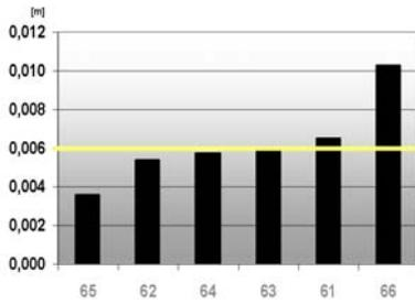
Table 3. Comparison between targets, topographically measured, and the same ones on the cloud of points after global registration
