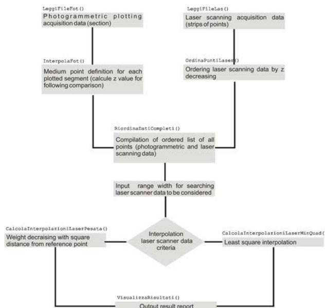
Figure 13. Flow chart of the program aimed at the comparison between the sections
