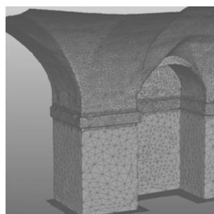
Figure 5. Curvature sampling. We can note the effects of the decimation: stronger in the regular surfaces
