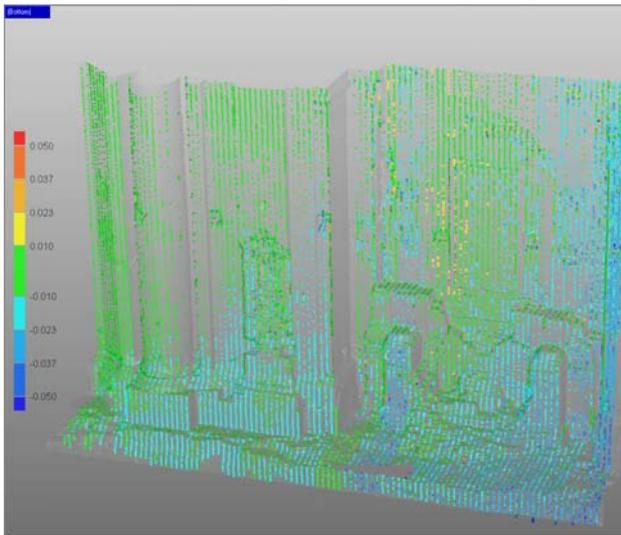
Figure 10. Graphic comparison between photogrammetric sections and laser scanning model. Residuals  $< \pm 2$  cm
