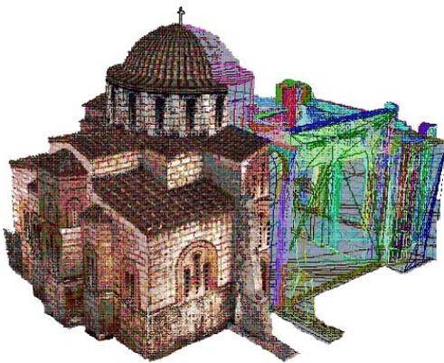
Figure 9: Orthophotos layered on the surface model
