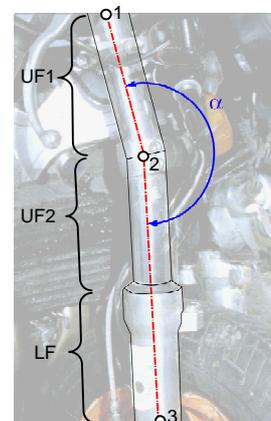
Figure 3: Bent off wheel fork
