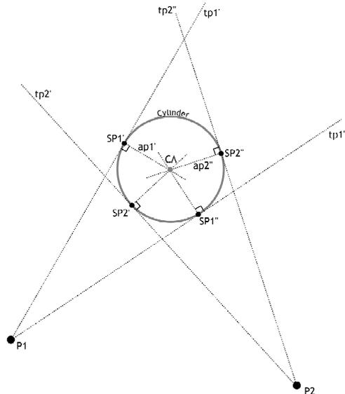
Figure 10: Modelling the fork cylinder axes
