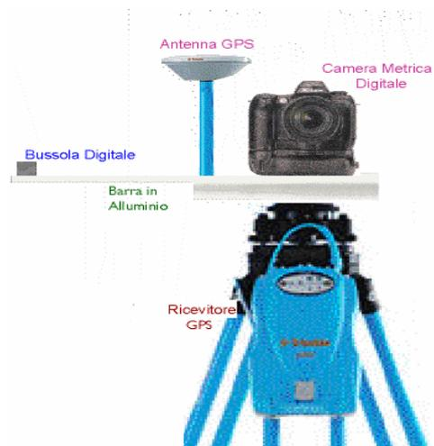
Figure 1. Diagram of the Mobile Mapping System “POLIFEMO”
