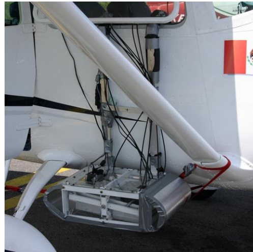
Figure 5: DCS Pro 14n in outside platform installation (© GeoSisA 2004).
