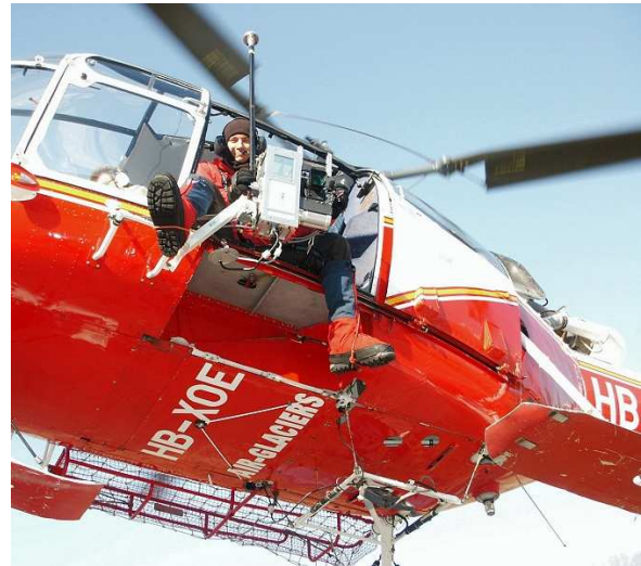
Figure 4: The system in action with Alouette III helicopter. The holder for supporting the system weight during transition flights is located under operator's right leg.
