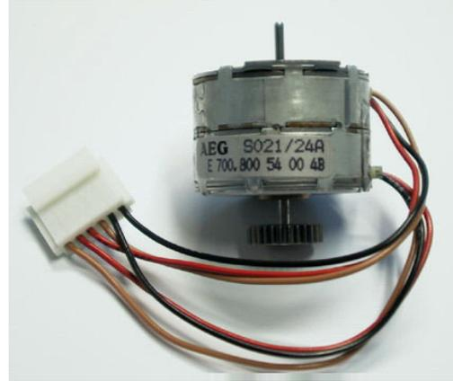
Fig. 1. The stepper motor
