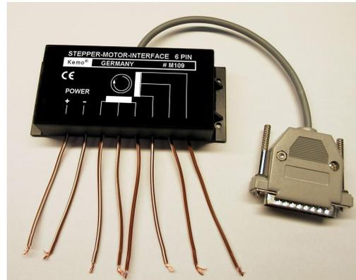
Fig. 2. The parallel port stepper motor interface kit
