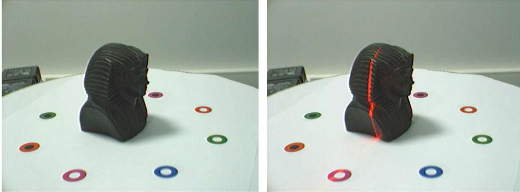
Fig. 3. The difference of the two images provide the points whose 3D coordinates are calculated
