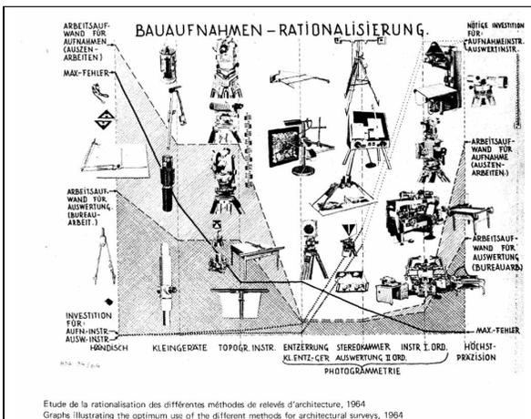
Figure 5: Foramitti's illustration of different documentation methods
