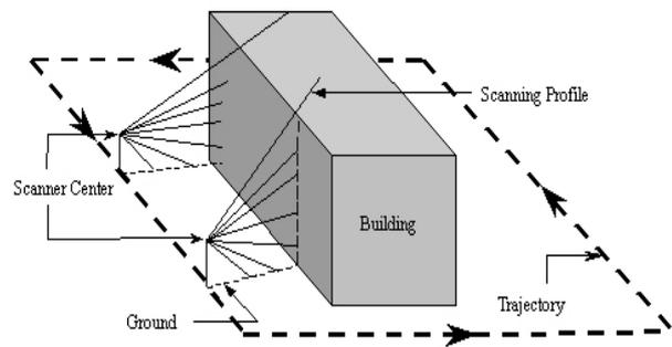
Figure 1: The principle of scanning a building object and other visible objects around the building
