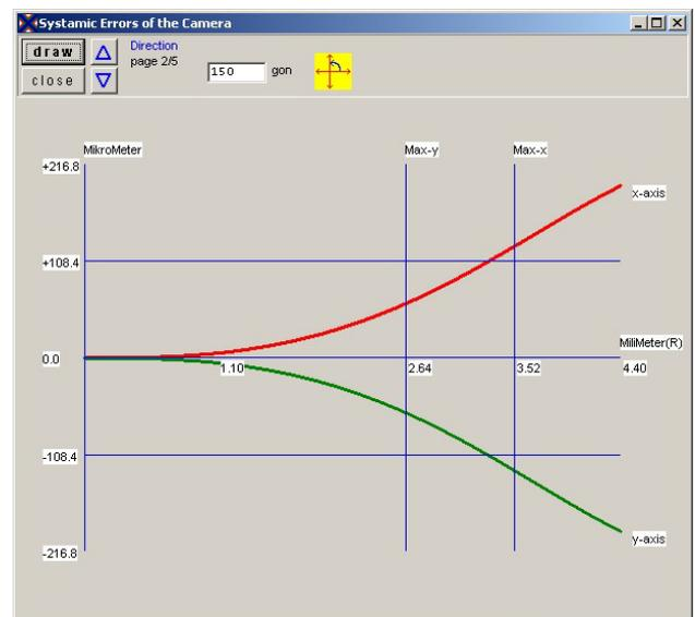
Figure 7. Total distortion curves along predefined directions (red: x-axis; green: y-axis)
