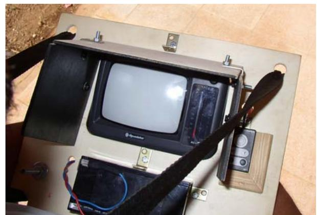
Figure 4. Ground control unit with monitor in the centre, remote controller on the right and battery for the monitor downside of the monitor
