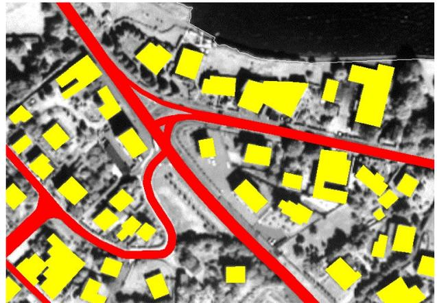
Figure 5 – Overlapping of the extracted vector layers to the IKONOS orthoimage patch.
