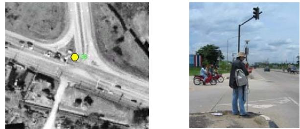
Figure 3. Left: A well-defined point on the image. Right: Corresponding point measured by GPS on the ground.
