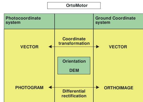
Figure 6. OrtoMotor coordinate transformation schema
