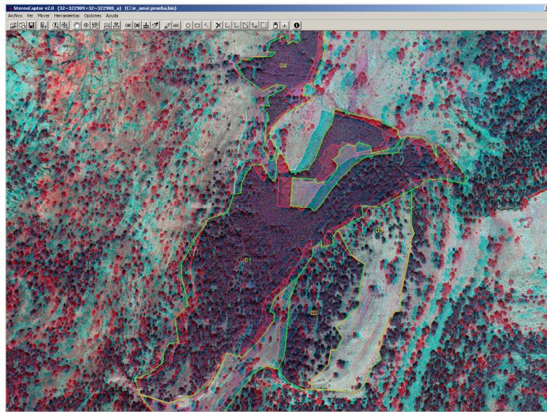
Figure 5. Superimposition vector information over infrared stereoscopic model (StereoCaptor tool)
