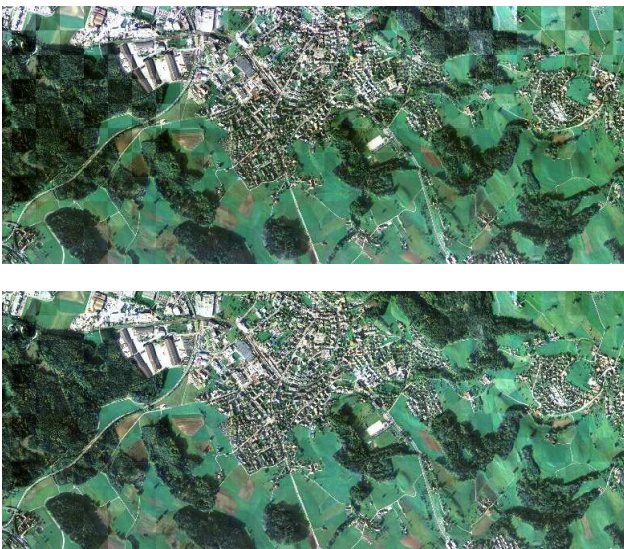
Figure 6. Image mosaics before (top) and after (bottom) BDRF correction. The mosaics each consist of two images flown in opposite direction (EW and WE) with the forward looking RGB lines of an ADS40. Dark forest shows a larger discrepancy after correction and should be modelled separately.
