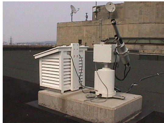
Figure 5. Sky Radiometer at Kanazawa Institute of Technology (36.53°N, 136.63°E)
