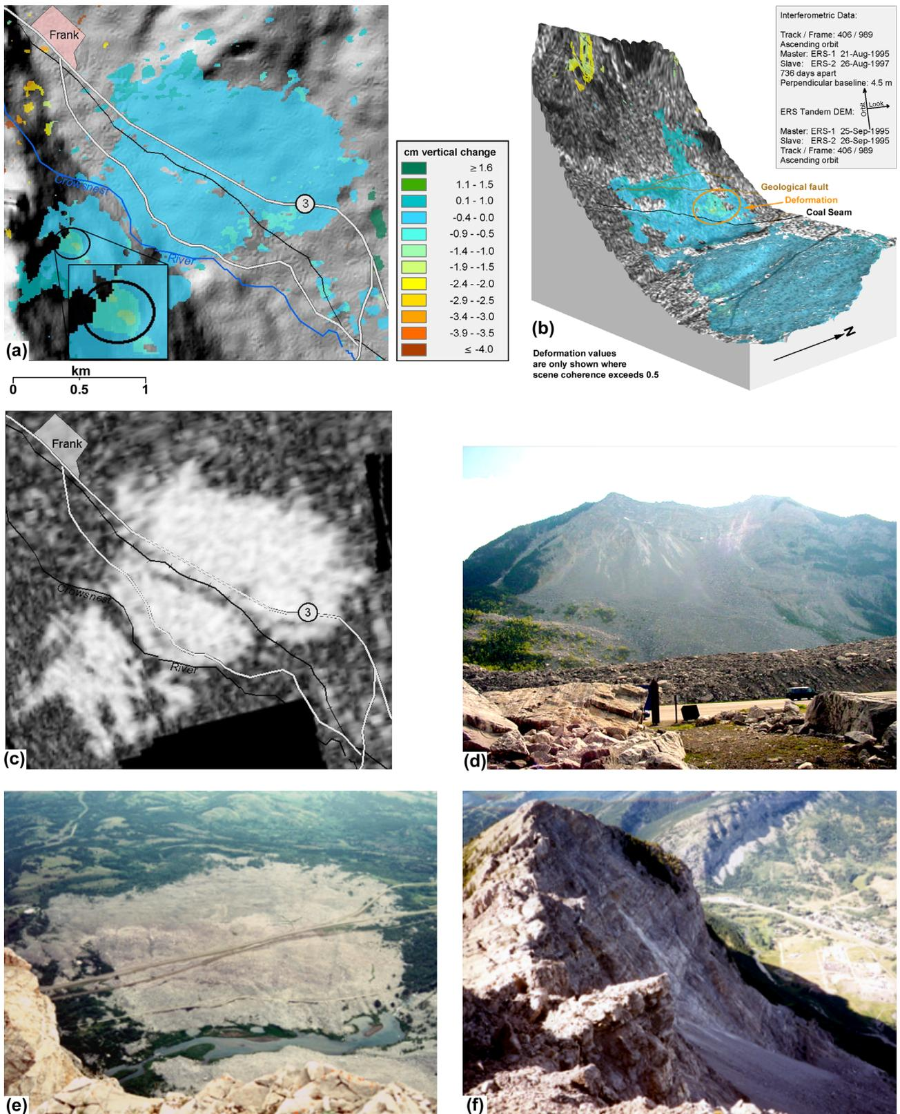
Figure 1. Vertical surface deformation map, generated from differential SAR interferometry (a). Result is draped over a high-resolution elevation model (b). Corresponding coherence image (c), and field photographs (d-f). The deformation is located towards the bottom of the slope, just above a coal seam.
