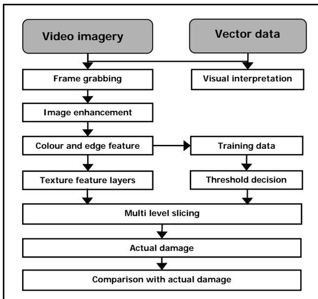
Figure 3. Damage assessment using video imagery
