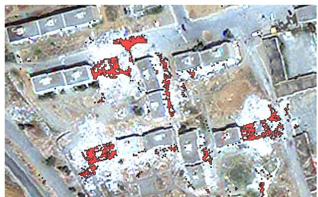
Figure 3. Boumerdes, change detection results by pixel-based classification.
