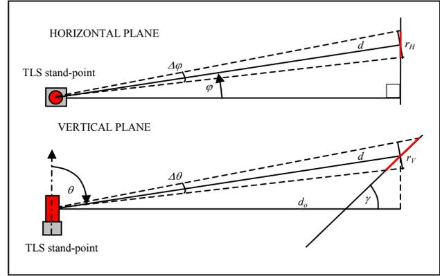
Figure 1: geometric scheme for computing footprints.
