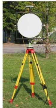
Figure2: reflective target for LR TLS applications with GPS antenna mounted
