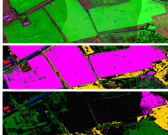
Figure 9: The image of the test area with variance in illumination (up) and the classification results of Spectral Angle Mapper (middle) and Maximum Likelihood (down).
