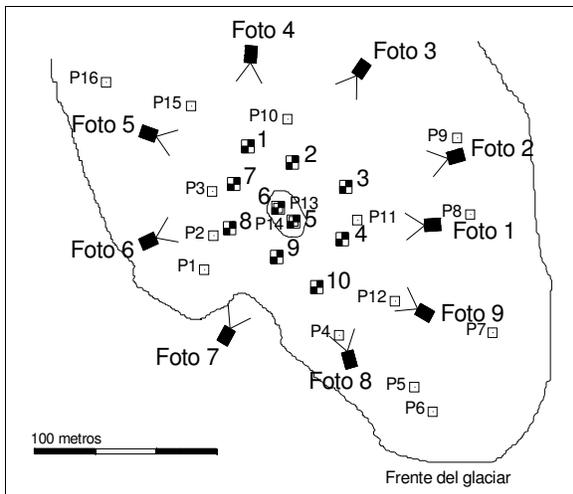
Figure 4. Scheme of the rods, control points or artificial signs of the photogrammetric takings.
