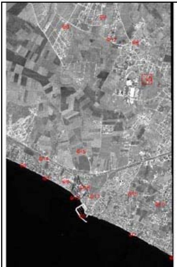
Figure 2. GCPs observed by GPS measurements in QuickBird image.
