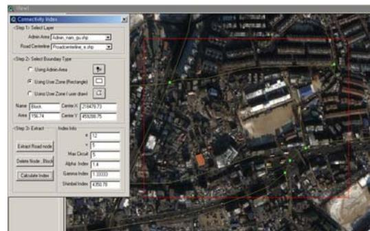
Figure 2. User interface of extraction extension program of Connectivity index with IKONOS imagery
