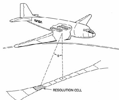
Figure 1. ESTAR radiometer on board P3 aircraft
