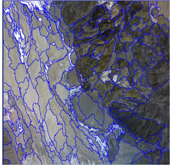
Figure 6. The third level of the multiresolution segmentation applied to the ASTER and DEM dataset.
