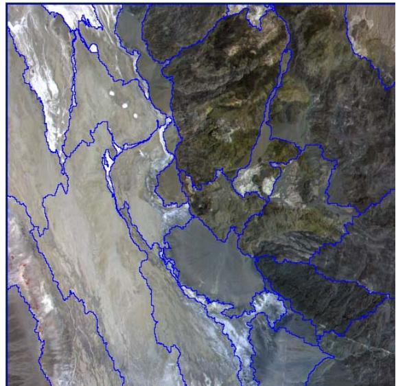
Figure 7. The fourth level of the multiresolution segmentation applied to the ASTER and DEM dataset.
