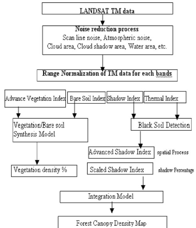
Figure 4. Flow chart of FCD Mapping Model
