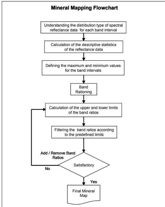
Figure 6. Flow chart of the mineral mapping technique.
